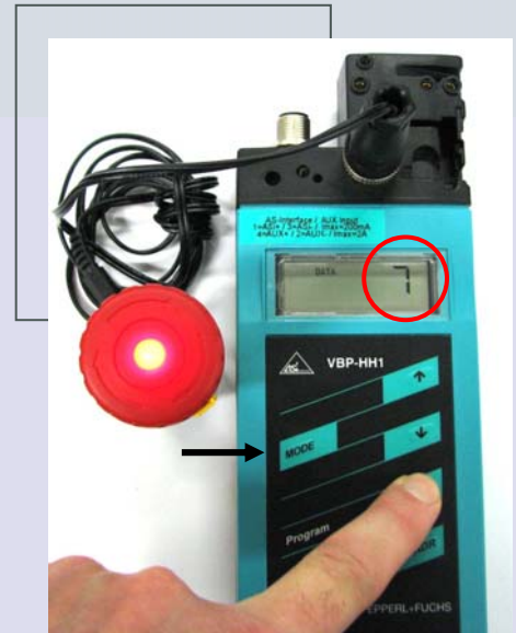
Press the „MODE“ button to switch into the menu „DATA“ for setting outputs.
